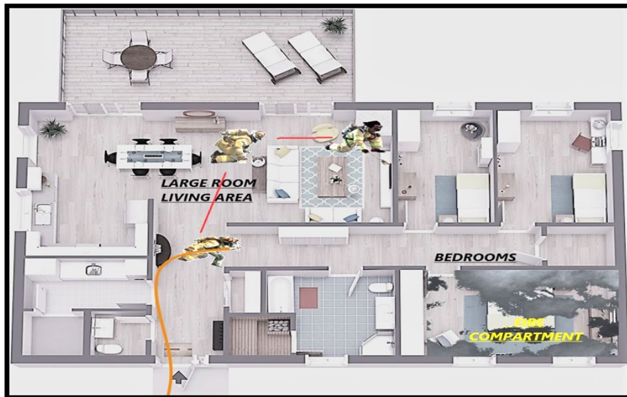
(FIGURE 11) AFTER THE INITIAL KNOCK DOWN IN A BACK BEDROOM, THE NOZZLE CAN BE PULLED BACK TO THE HALLWAY ENTRANCE TO SHIELD THE SEARCHING FIREFIGHTERS FROM ANY SUDDEN BURSTS OF FLAMES AND ENABLE CLEAR COMMUNICATION WITH THE OIC AS THEY SEARCH THE LIVING AREA.
